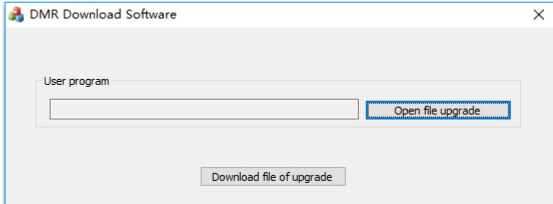
2. Connect the radio to the computer with the programming cable, press and hold PTT + SK1 when turn on the radio, the radio will go into update mode and the Rx/Tx signal light will flash green and red.
